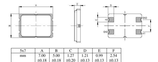
NOTE: For proper electrical performance of crystal resonator, GND pads should be electrically connected to ground in the final application.
